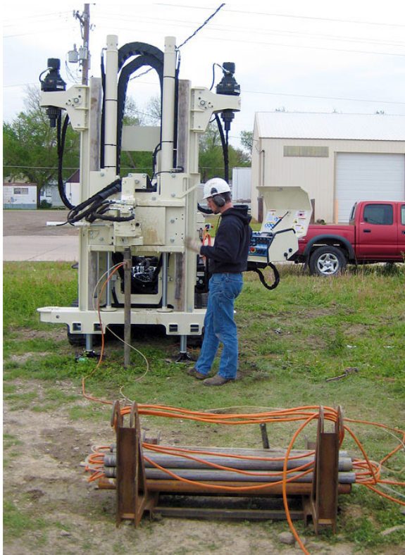
Trunk line threaded through drill rods
